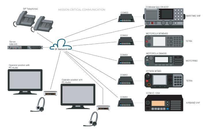
IHM IP FLEXIBLE ENTERPRISE is a costefficient and highly reliable communication solution built of standard modules. The solution is designed for companies and organisation, which needs the highest flexibility in numbers of radios / base stations, operator positions and functionalities.
